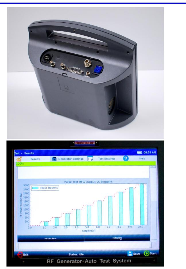
This screen shot shows the performance of this generator as an average of stored data from previous tests, the dotted line represents an ideal result. The most recent test shows a change in RF output vs. setpoint.
